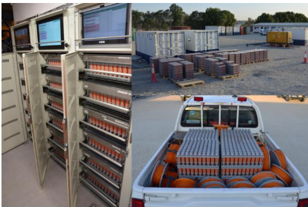
Figure 2 - Top right: the nodal central system in camp with its three core units inside 20ft standard containers. In the foreground we see 35,000 nodes (out of the 50,855 nodes used) prepared for deployment. Bottom right: 1500 nodes on a back of a pick-up truck including recovery strings. Left: downloading and charging racks capable of turning around 20,000 nodes per day.
